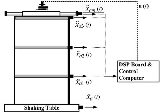
Figure 5. Experimental setup of a three degree of freedom model
