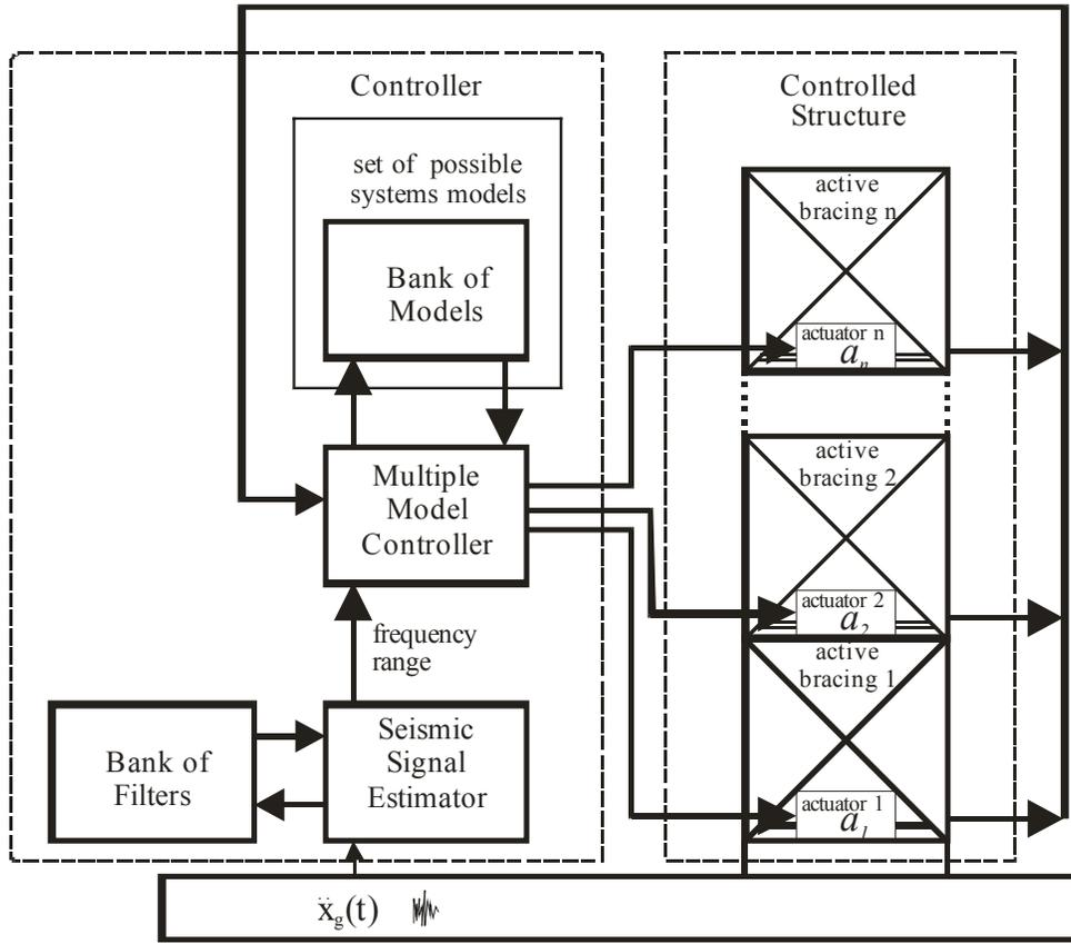
Figure 1 Multiple model seismic structural control system
