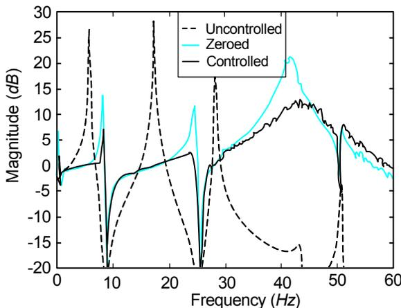
Figure 6. Comparison of uncontrolled zeroed and controlled transfer functions: ground acceleration to the first floor absolute acceleration.
