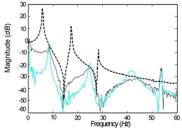
Figure 7. Comparison of uncontrolled zeroed and controlled transfer functions: ground acceleration to the second floor absolute acceleration.
