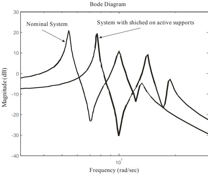
Figure 3 Frequency - magnitude characteristics of the nominal system with removable cross braces.
