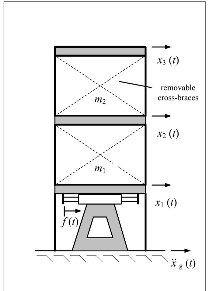
Figure 2 Experimental setup of active bracing control system
