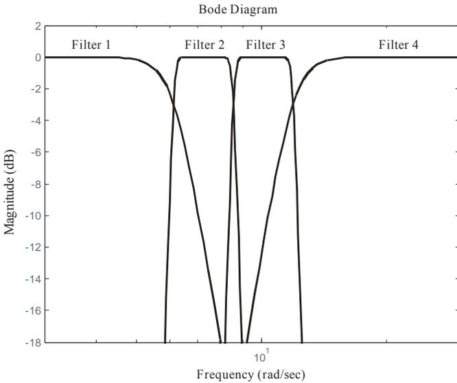
Figure 4 Frequency - magnitude characteristics of the proposed Butterworth filters.
